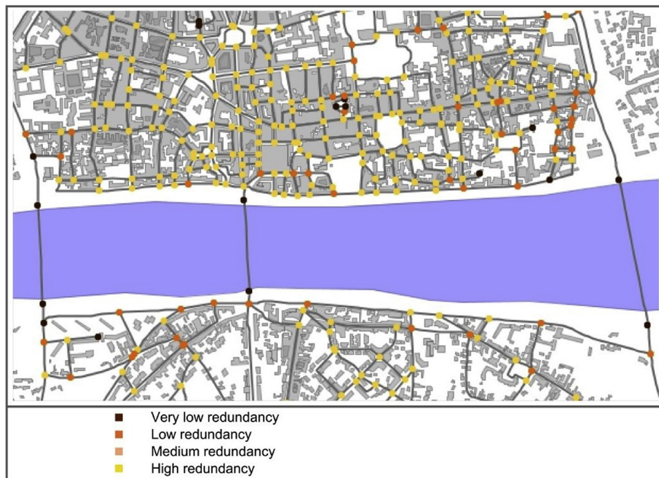
Fig. 7. Orleans (France) road network redundancy analysis shows the weak redundancy of this network close to bridges (source: Lhomme et al., 2013).
